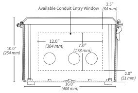
THE CONTROLS ENCLOSURE IS NOT PRE-DRILLED FOR ANY CONDUIT ENTRIES. Actual conduit size, qty, and locations are determined at the discretion of the installer.
