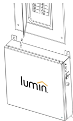
1. Mount Lumin Smart Panel (LSP) near main panel.
