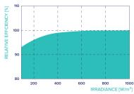
Typical module performance under low irradiance conditions in comparison to STC conditions ( $25\,^{\circ}$ C,  $1000\,\text{W/m}^2$ ).
