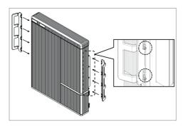
1. Fix the lift handles to the hex-socket screws on the rear (marked position) of both left and right sides.
