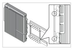
3. Mount the battery pack to a wall bracket's "U" shape clip using the support by lift handles. Remove the lift handles.
