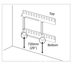
2. Mount the wall bracket to a wall. Tighten the screws, ensuring that they are horizontally driven into the wall. (Must be installed with recommended clearances(720mm[29"]) on the edge of the wall bracket as shown in the figure)
