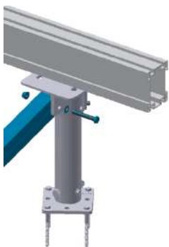
Install the SunBeam Rail on the Pipe Caps
