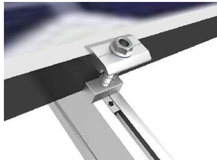
Grounding Mid Clamp to Rail. The universal mid clamp accommodates module frames from 31 to 50mm.
