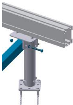
Install the SunBeam Rail on the Pipe Caps. See SunBeam on page 37.
