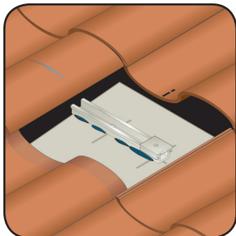
Step 7: After bolting the base to the roof, slide the upper carriage into the correct position under the crown of the tile. For Flat tile, slide the upper carriage near the middle of the tile.
