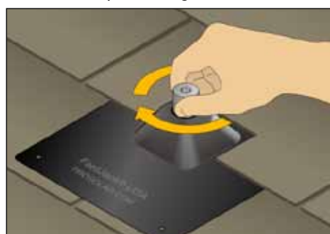
Step 6: Tighten FastJack® post into base
