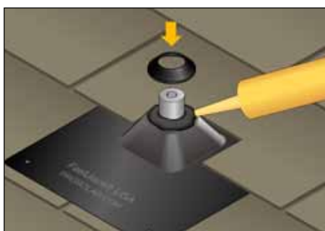
Step 7: Apply sealant (Geocel 4500) and compress with Aluminum collar.
