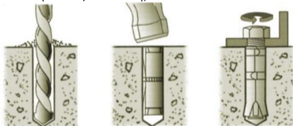
Figure 2.6 – Drilling holes for mounting hardware
