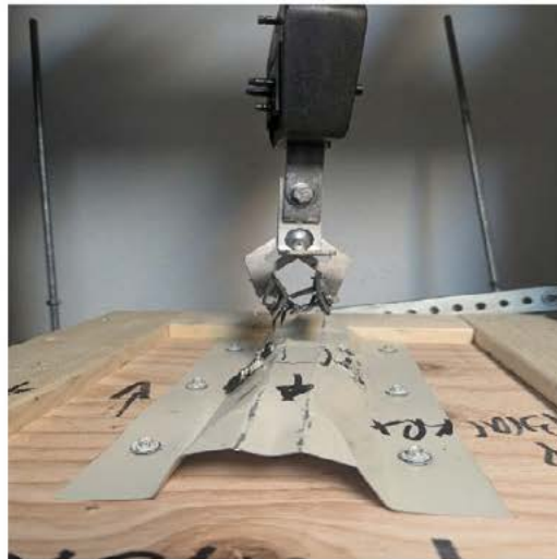
The mounting arms fasteners pulled out of the sheet metal
