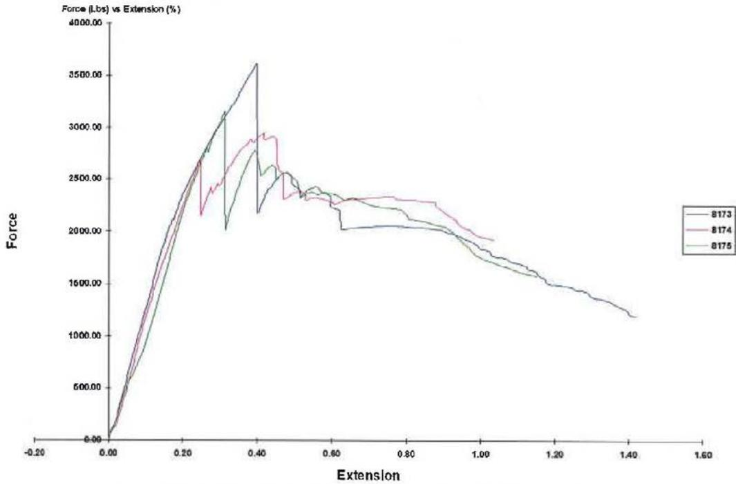
Figure 1. Test 8173, 8174, 8175 tensile load vs. displacement curve.
