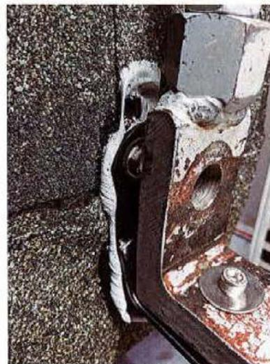
**Figure 4c.** Bolt failure mode.
