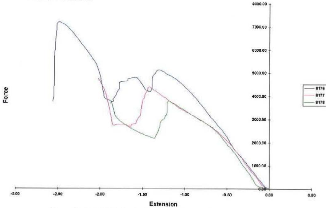
Figure 2. Test 8176, 8177, 8178 shear load vs. displacement curve.
