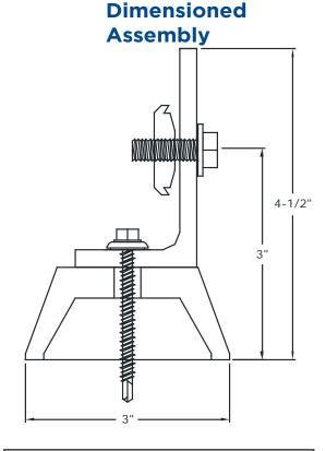
Tek Screw For Steel Roofing Members, Lag Screw For Wooden Rafters
