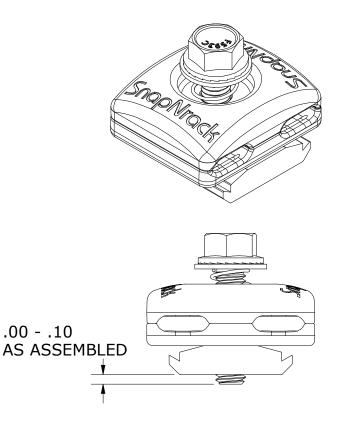
\*THIS ASSEMBLY WORKS WITH TRUNK CABLES OR OTHER WIRES 0.21" - 0.45" IN DIAMETER
