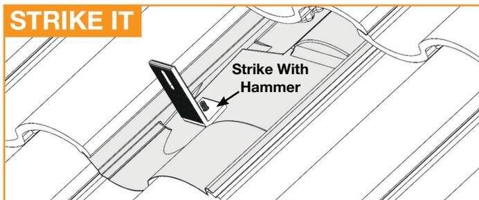
Insert the lag bolt with bonded washer through the base into the pilot hole. The base can be installed parallel or perpendicular to the rafter.
