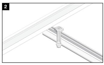
Place module on rails (module cells not shown for clarity).
