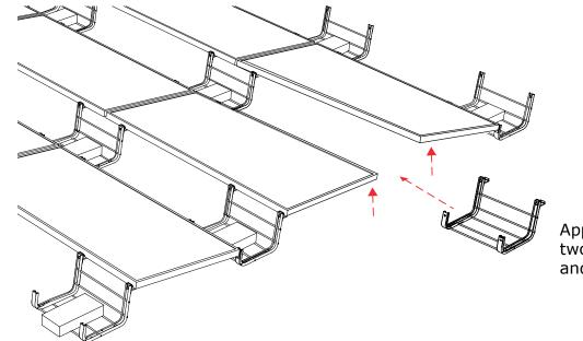
Apply gentle, even uplift on the two adjoining module frames, and slide bay into place.
