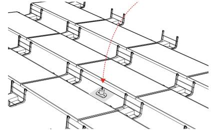
Note: Peel'n'stick type flashing not recommended for this. Remove ballast from the bay, and possibly surrounding bays.
