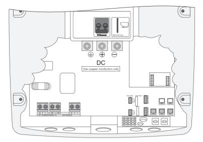
Use conduits to install the cables on the DC side and on the AC on the Sunny Island. Conduits ensure the dust- and water tight mounting of the lines on the enclosure and also serve as a strain-relief of the lines at the connection. Close all unused openings in the enclosure using the appropriate filler-plugs.
