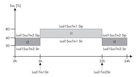
The figure shows an example of the settings if the load shedding function at night is to be avoided as much as possible. From 6:00 a.m. to 10:00 p.m. the load shedding is activated for a state of charge (SOC) of 40%, at nighttime (from 10:00 p.m. to 6:00 a.m.), however, the state of charge of the battery is allowed to go down to 30% before the load shedding contactor is activated.
