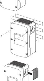
oxdot The Sunny Island is mounted using the wall mounting bracket.
