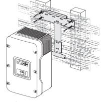
If two or more Sunny Island inverters have to be installed, mount the inverters on two studs each in order to get better cooling. Make sure that the wall where you intend to install the Sunny Island is vertical and can carry the weight of the Sunny Island (139 lbs, 63 kg) on a long-term basis.
