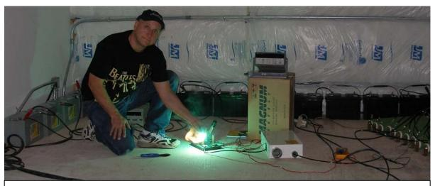
Pictured above, boB breaking 165VDC at 99 amps for the first test. This arc is the same arc that our little breaker must deal with internally. The arc is not only blinding, but also extremely hot. Pretty amazing huh! I also discovered the hard way that getting shocked with 165VDC feels pretty much the same as getting shocked with 120VAC.
