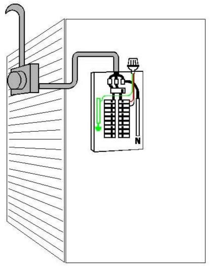
In a utility connected home, one of the most vulnerable points of entry is the service entrance panel. All house wiring connects to the service entrance panel and therefore everything plugged in is at risk. The MidNite SPD300 provides protection against near lightning strikes up to 100,000 amps of surge current. Hooking up to the service entrance can be done in a few different ways.
