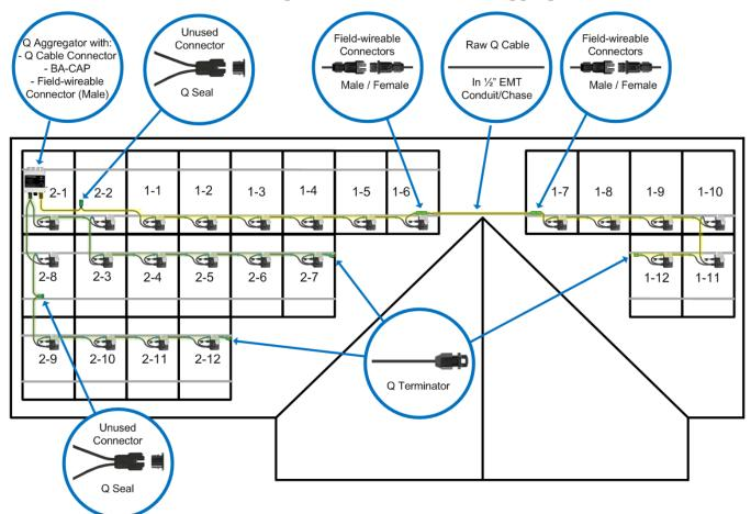
Scenario 3: 24 Module, Two Strings of 12, Terminated at Q Aggregator
