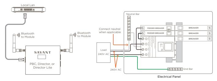
HELPFUL! The diagram shows an electrical panel that doesn't contain a plug-on neutral bus bar. However, both plug-on neutral and nonplug-on neutral panels are supported.
